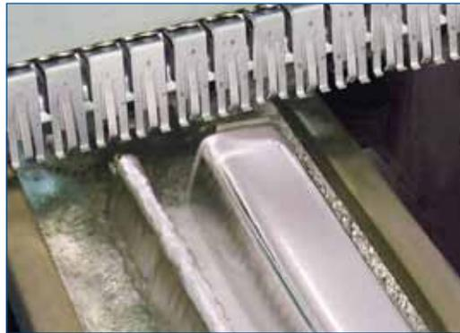
*Fig 1: Turbulent wave (left) and Laminar wave (right) in same system*
