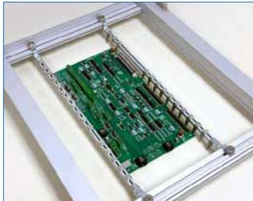
*Fig 7: Adjustable pallet holds multiple board sizes for fast changeover*
