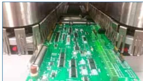
**Pros:** Good support for odd-shaped boards or thin boards that could warp otherwise; can be customized to hold unusually shaped boards, or multiple boards; very easy to maintain pallets and fingers because everything can be done outside
