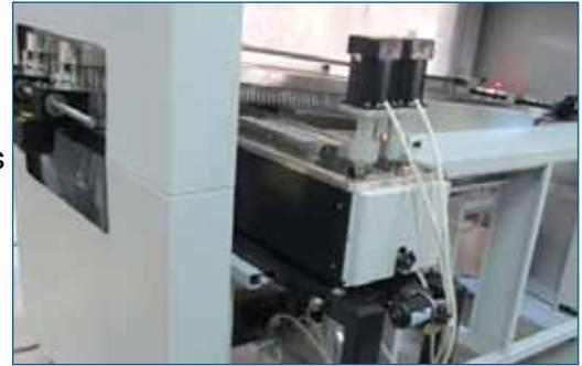
*Fig 12: Rollout solder pot*
