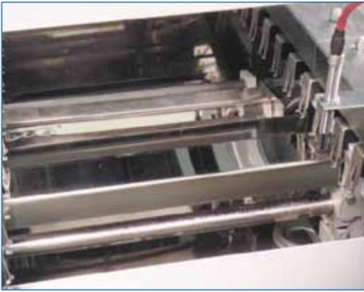
Fig 9: Flux air knife
